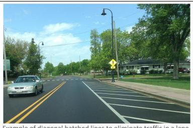
Example of diagonal hatched lines to eliminate traffic in a lane.
